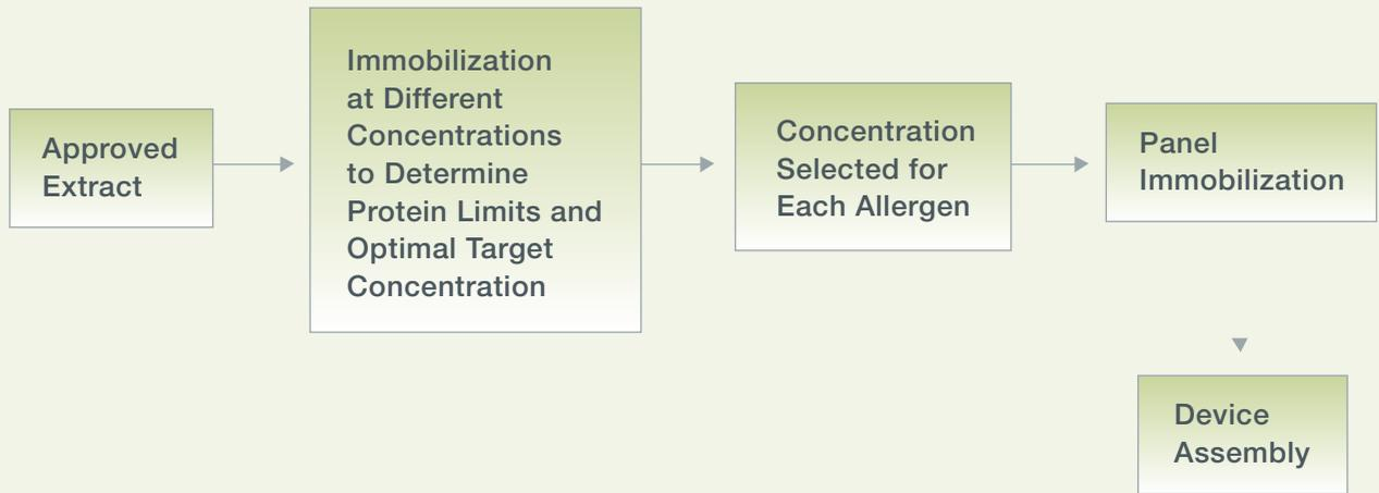
Fig. 8 | Summary of the Manufacturing Process for OPTIGEN
