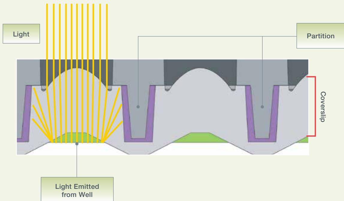
Fig. 4 | Cross-Section of the Partition and Coverslip for OPTIGEN
