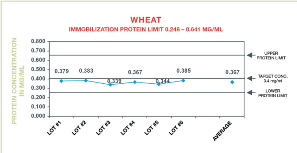
Fig. 9 | Process Control Chart for the Immobilization of Wheat over Six Production Lots
