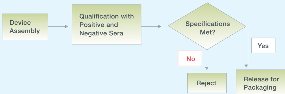
Fig. 10 | Summary of the Qualification Procedure for OPTIGEN
