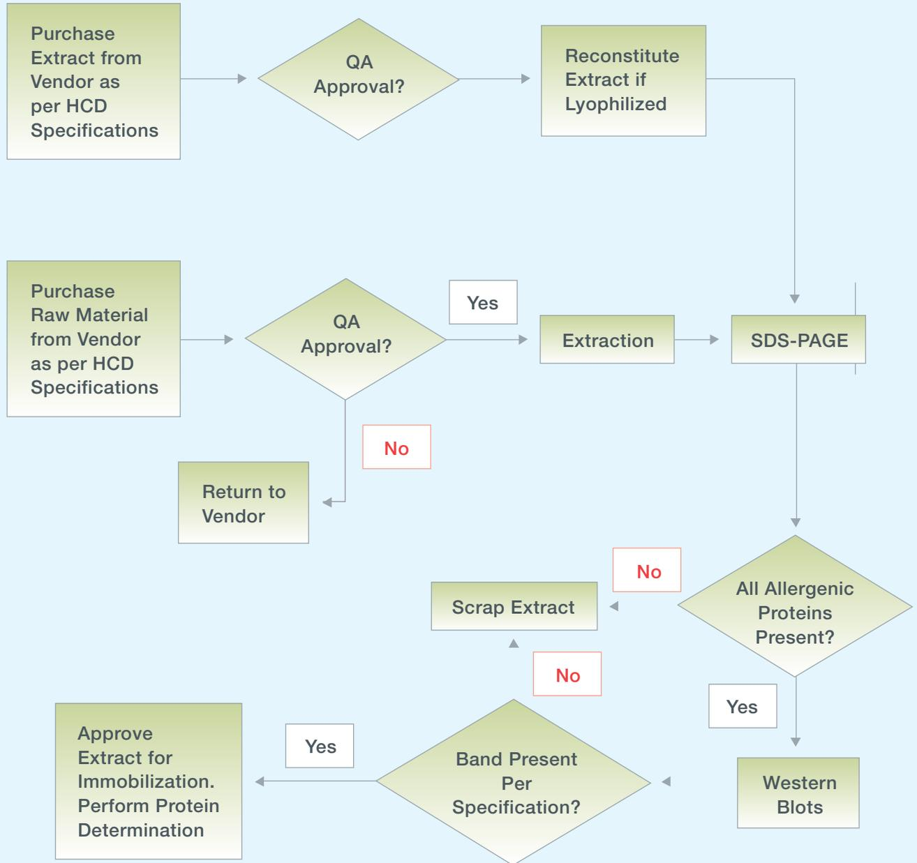
Fig. 5 | Process from Raw Material to Extract at HCD
