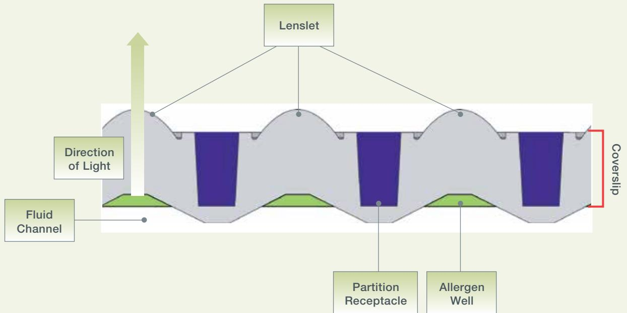
Fig. 3 | Cross-section of the Coverslip for OPTIGEN
