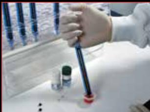
Fig. 8 | Draw photoreagent into pettes
